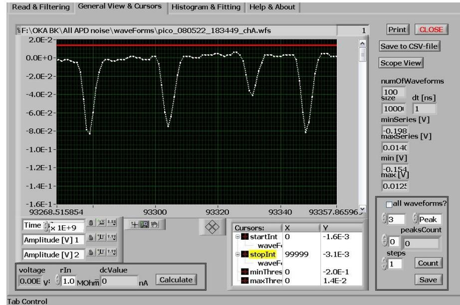
As an example the signal shapes obtained with 1 mm CPTA APD is shown. Noise pulse width was ~8 nsec at the base line with rise time of ~2 nsec. Time grid has 20 nsec pitch with 1 nsec between samples.
