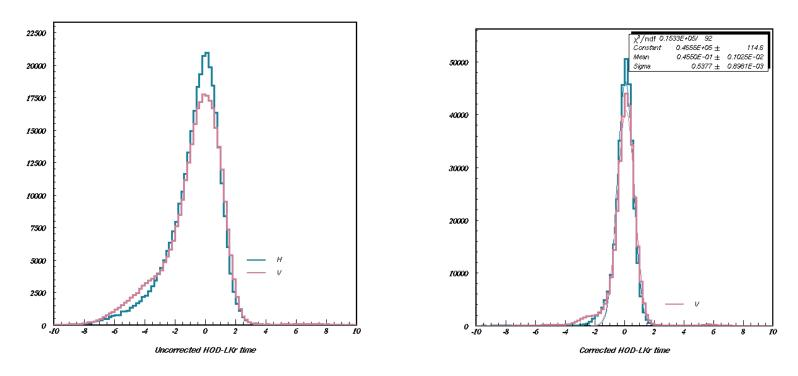
CHOD-LKr time: the time resolution changes applying the correction with the crossing point from 3-4 ns to 540 ps (1 trk, 1 cluster, 1 electron, 2 chod, 2 chod\_neut)
