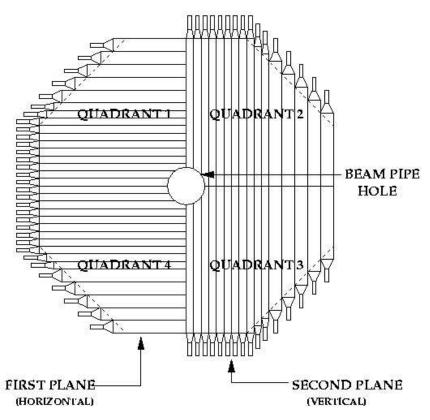
The **CHOD** is composed by 128 scintillator's slabs, subdivided in 2 planes, with slabs oriented orthogonally (H and V) • Each slab is 2 cm thick, 6.5 to 9.9 cm wide and 60 to 121 cm long
